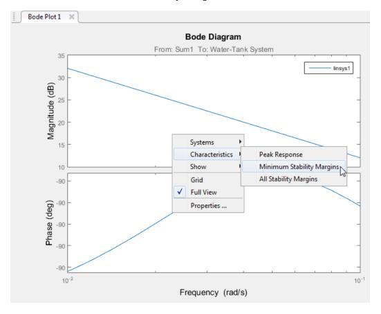
The Bode plot displays the phase margin marker. To show a data tip that contains the phase margin value, click the marker.
