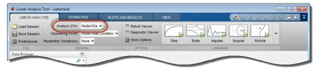
To linearize the model using the specified analysis points and generate a Bode plot of the
