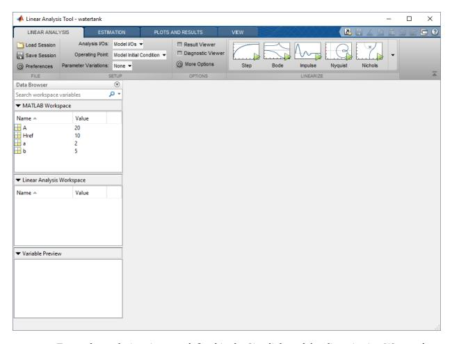
To use the analysis points you defined in the Simulink model as linearization I/Os, on the  $\bf Linear\ Analysis\ tab$ , in the  $\bf Analysis\ I/Os\ drop\ down\ list$ , leave  $\bf Model\ I/Os\ selected$ .
