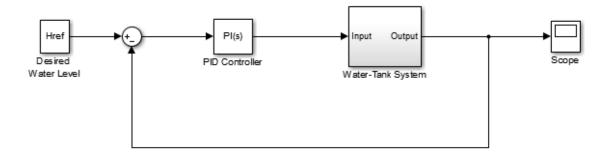
The Water-Tank System block represents the plant in this control system and includes all of the system nonlinearities.
