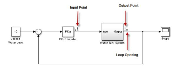
For more information on defining analysis points in a Simulink model, see "Specify Portion of Model to Linearize in Simulink Model". Alternatively, if you do not want to introduce changes to the Simulink model, you can define analysis points using the **Linear Analysis Tool**. For more information, see "Specify Portion of Model to Linearize in Linear Analysis Tool".
