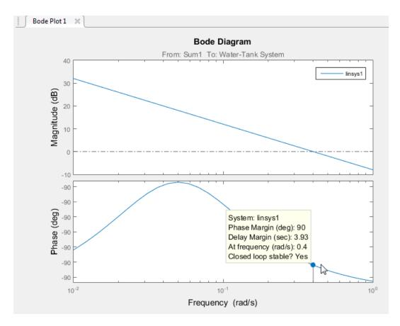
For this system, the phase margin is 90 degrees at a crossover frequency of 0.4 rad/s.
